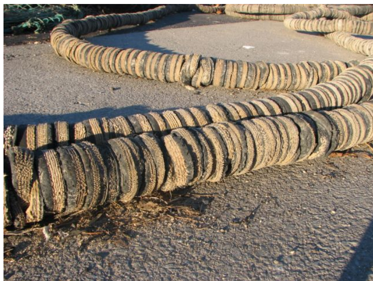
Figure 3 – Ground cable with cookies
